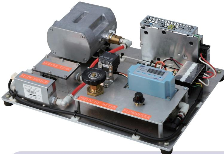
AIRTRONICS controls FC blowers to provide flow volume adjustment, and insure constant flow output when inlet supply pressure fluctuates.
